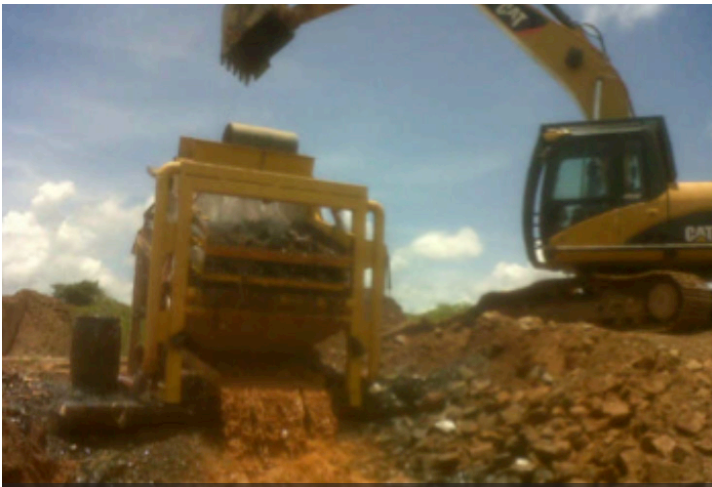
Wash Plant operating
