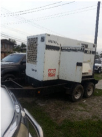
85 KVA PLANT GENERATOR
